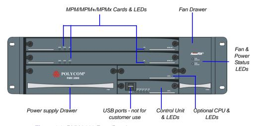
Figure 1-1 RMX 2000 Front Panel
